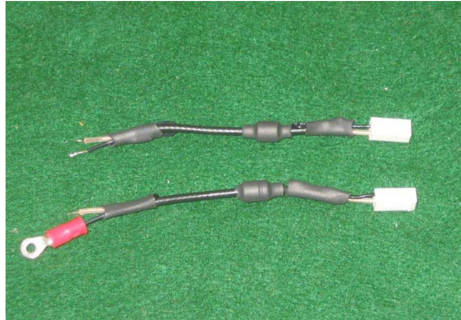
Illustration 2: Completed RF cables.
