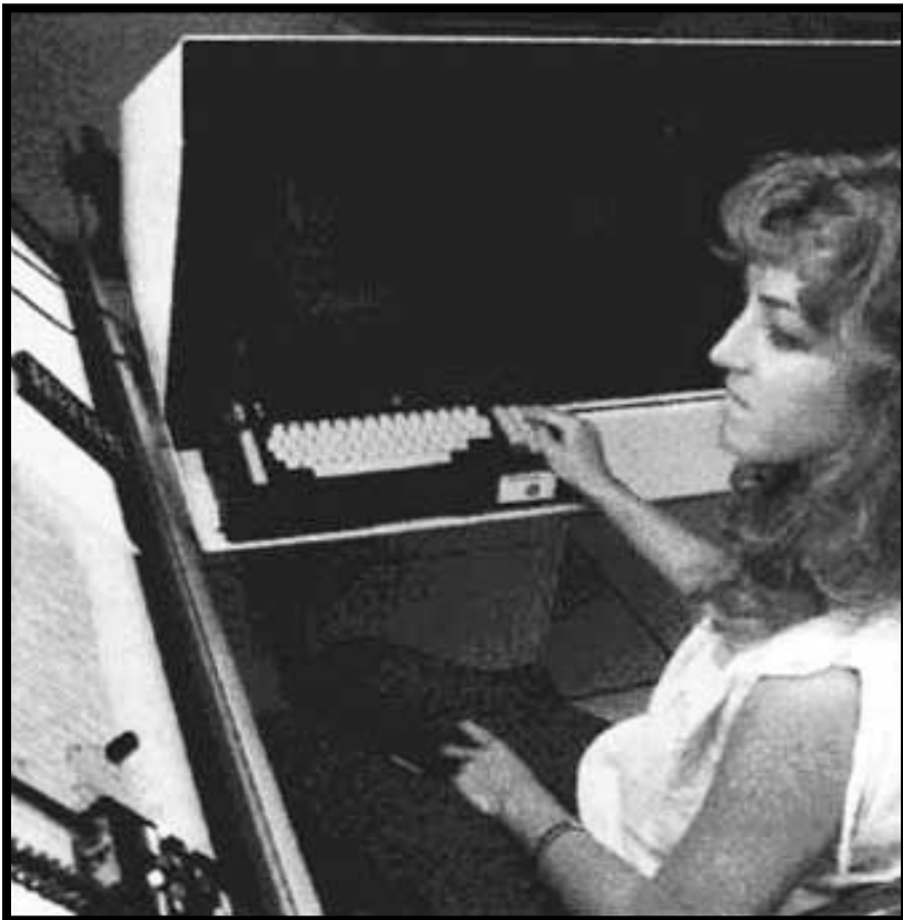
Photo 4: Digitizing. Computer aided design (CAD) technician Lisa F. enters a cell layout into the data base. The cursor on the light table is used to transfer precision measurements to the computers. An already digitized cell is shown on the video display.
