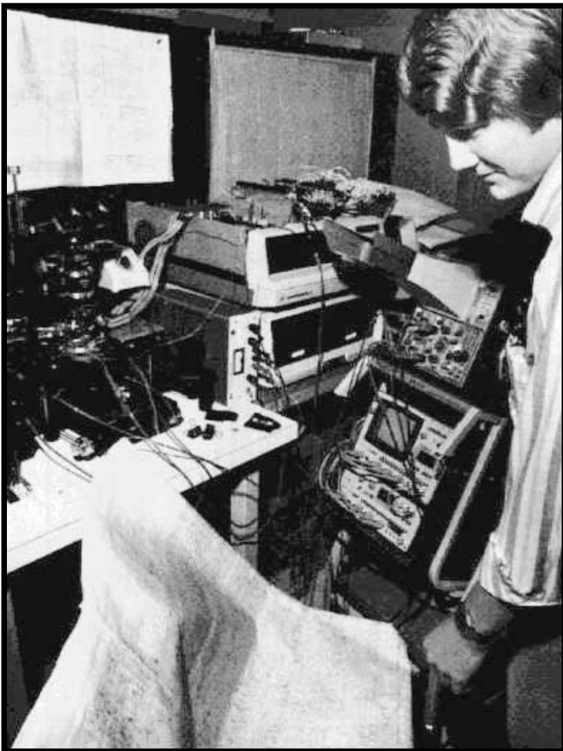
Photo 5: First silicon engineering analysis. Logic and circuit design engineer Bob Thompson tracks down a weak node in the first batch of 6801 chips. The 6801 die is packaged, but not sealed, so that internal nodes may be probed while in operation. Viewing through a microscope, a probe can be placed at critical points equivalent to the layout plot. The chip itself is running a modified EXORcisor system, and the scope actually displayed an internal signal with excessively slow rise time.
